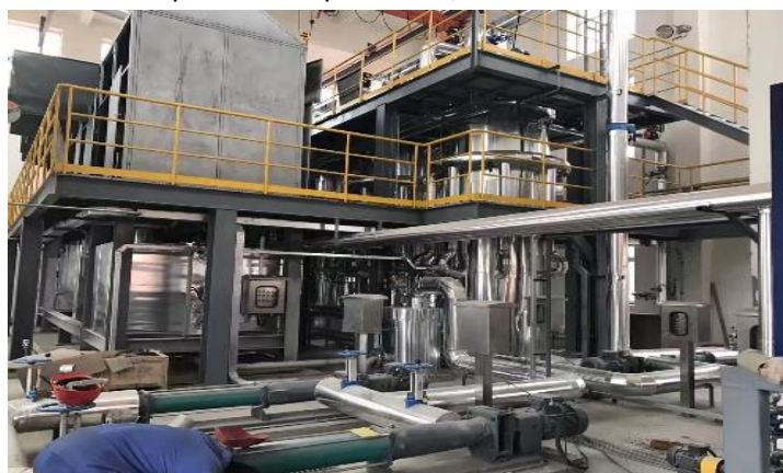
Figure 16. Use of reclaimed water in thermal hydrolysis processes at the Mudanjiang First Water Plant of our Northeast China business unit.
