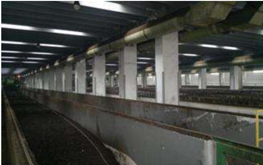
Figure 20. High-temperature aerobic fermentation chamber at the Xinxiang City Sludge Treatment and Disposal Project.
