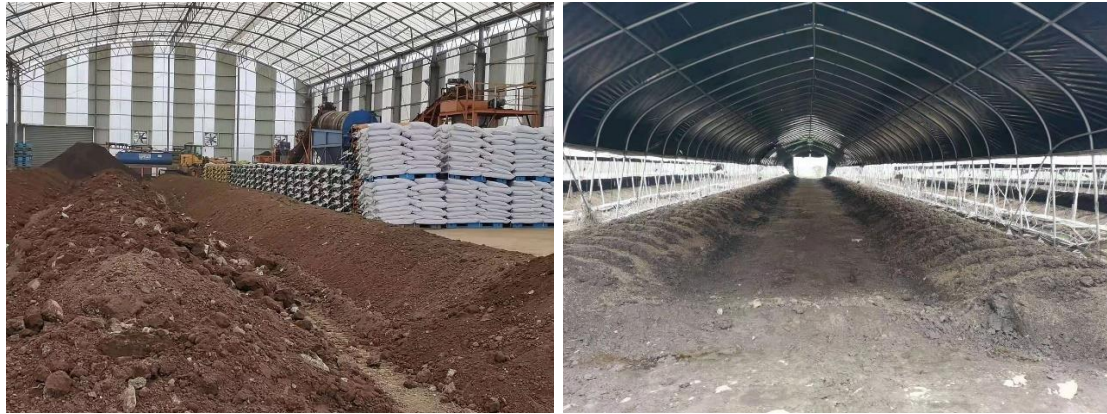
Figure 9 At the Wuhan City Huangpi District Panlongcheng WWTP Project 1 st Phase, the sludge is fermented at high temperature and digested by earthworms to form earthworm manure and earthworm products, which are sold to the local agriculture bureau and community.
