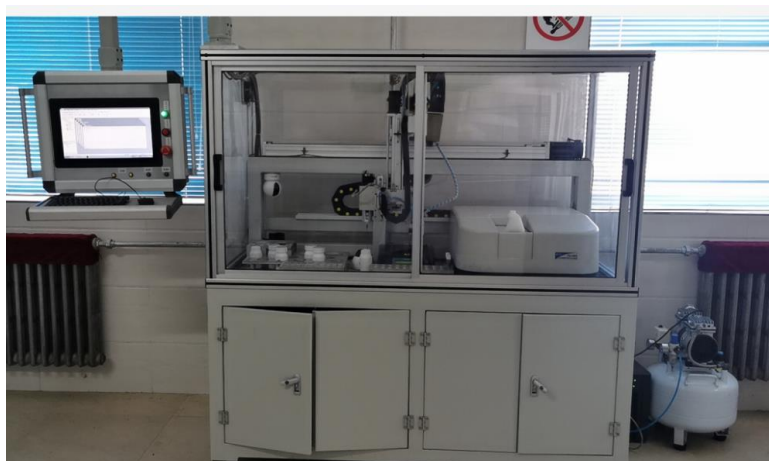
Figure 8 Laboratory robots used at our WWTPs.
