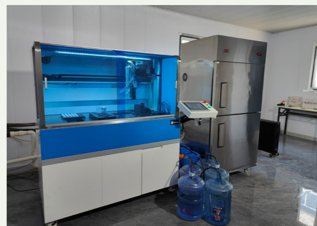
Precision dosing systems for carbon sources and phosphorus removal chemicals have been used in our project companies
