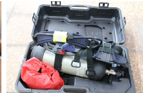
Protective clothing and activated carbon filter canister (left) and positive pressure respirator (right)
