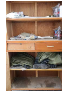
Protective clothing and activated carbon filter canister (left) and positive pressure respirator (right)
